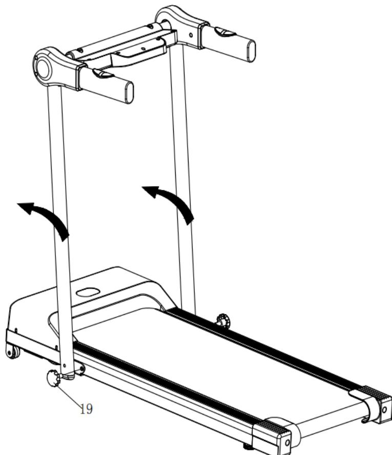
**STEP 2:** Fold up the handles. Use the M8x16 screws (10) and washers (9) to attach the handles to the front supports as described in the picture below.
