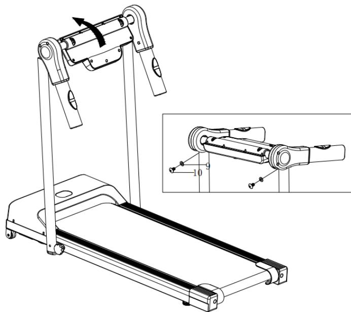
**STEP 3:** Fold up the console and secure it with the M8 handwheels. Insert the safety key (14) on the console, now you can start the machine.
